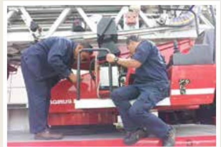
Pembaikan 'computer control' bagi jentera Turn Table Ladder (TTL) Repair of computer control for Turn Table Ladder (TTL)
