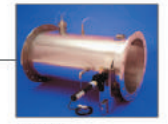
Duct insert Fitted into exhaust ducts of dynamic test methods. This houses gas temperature and mass flow probes and smoke measuring hardware
