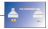
Furniture calorimeter Used to measure heat release and mass loss from furniture
